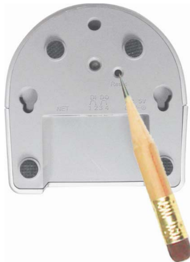
Figure 3-24: Stick on the reset button to set to the factory default
