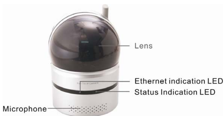
Figure 2-1: Major components in the front panel
