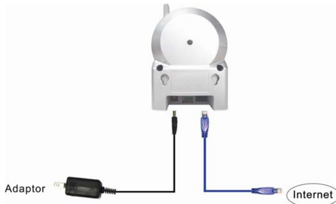
Figure 2-3: IP CAM connection diagram.
