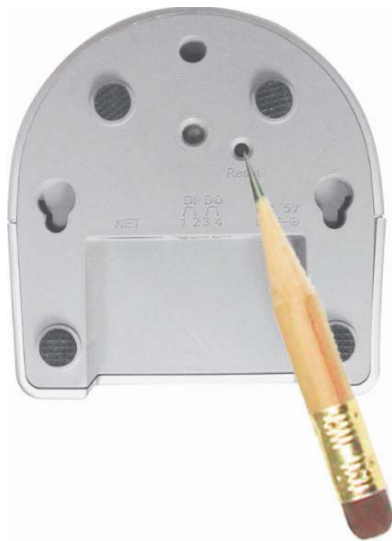
Figure 3-27: Stick on the reset button to set to the factory default
